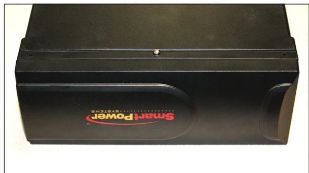
Place the cover back in and secure it with the screw located at the base of the UPS. Finally, plug all your equipment back to the UPS and turn UPS on by pressing the On button.
